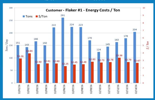
The energy costs per ton\* and temperature of the steam chest (at the conductivity sensor rods) are shown above and below, respectively. All graphical and tabular data is stored on a secure cloud drive that can be accessed by customer approved users.
