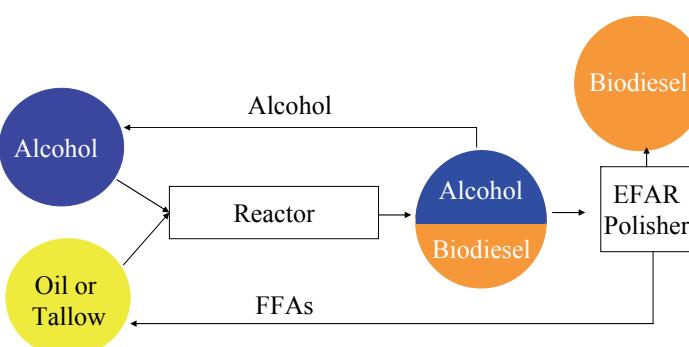
Figure 1. Schematic Diagram of the Patent Pending McGyan® Biodiesel Production Process Developed at SarTec®.
